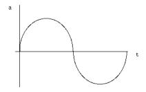
High and low pressure alternates at regular intervals, resulting in a simple periodic waveform (in this case, a sine wave). The length of the wave, 1/440 sec., also tells us the frequency indirectly. Since there are 440 cycles of pressure every second, we know the frequency is 440 Hz. The indicated amplitudes (1 and -1) simply indicate an arbitrary maximum and minimum.
