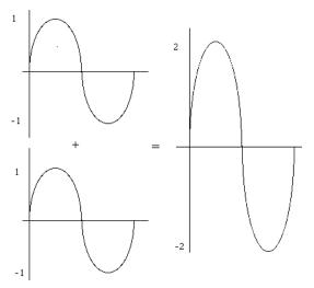
If we add a second wave at the same amplitude and frequency and begin both waves at exactly same time, they will reinforce each other and the result will be a doubling of amplitude. These waves are said to be 'in phase.' We can delay the onset of one wave, though, and
