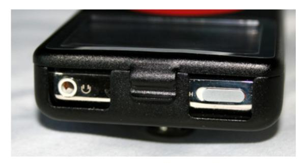
Shows access to hold switch and headphone jack, as well as clip holding the case together.
