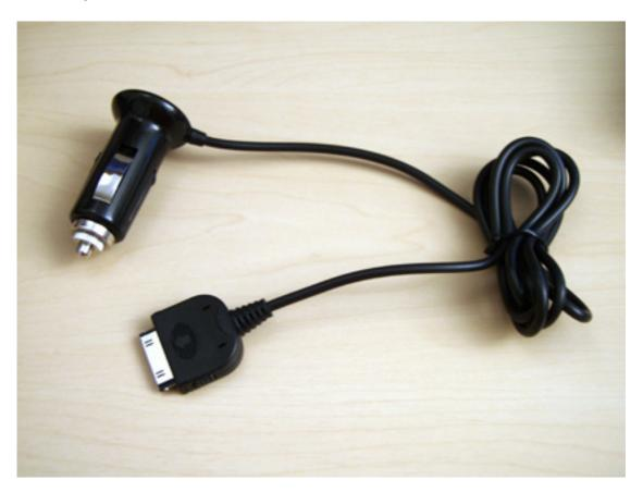
Most significantly, a considerable amount of force is required to insert and remove the charger's plug—a lot more than other chargers I've used. This overly tight fit is not required for the plug to stay in place. It's a good thing the end of the plug is flared so as to provide something to grip firmly while yanking it out of a power port. It's very much needed.
